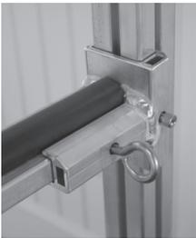
Install (1) allen bolt, (1) eye bolt and (2) brass nuts onto each of the (4) arm brackets. Loosely install the allen and eye bolts onto the arm brackets (**do not tighten them**).
