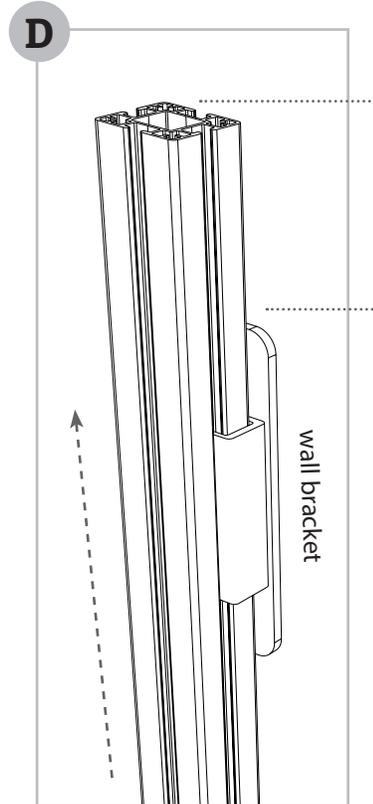
*Slide upright bar about 6" above wall bracket - this will allow you to install lower bracket in the proper position in Step 4.*
