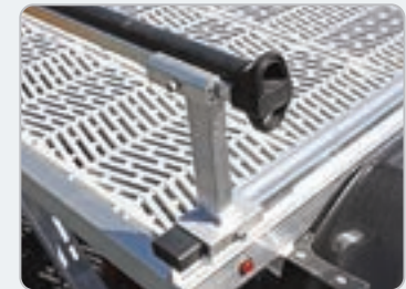
Load bars with custom end caps with built-in tie-down loops & vinyl hull guard included
