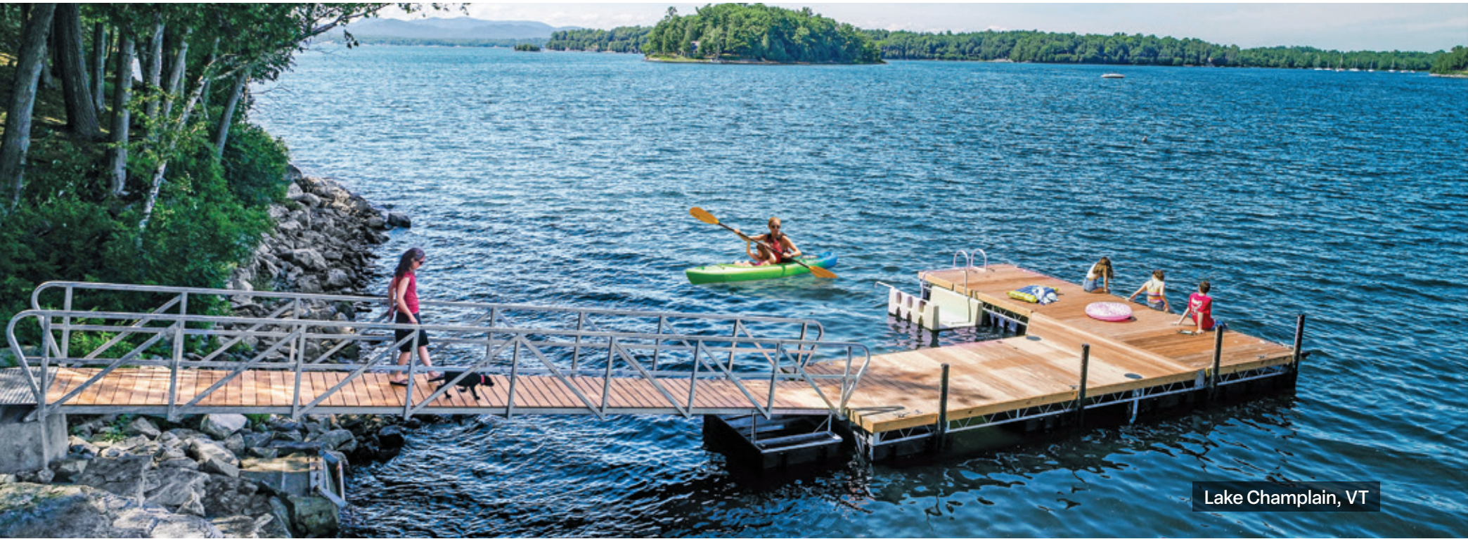
Above: Steel truss floating dock and gangway with Ipe decking. Below Left: Steel truss floating dock with Ipe decking. Our Mega Dock is used as a transition for a site that has high spring water levels. Below Right: L-shaped floating dock with WearDeck decking.
