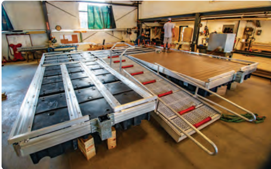
Above: Commercial launch getting final decking installed in our final assembly shop.
