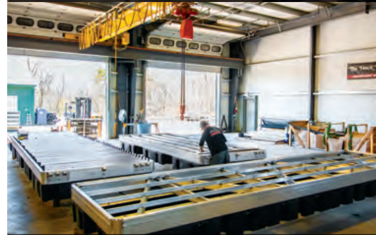
Decking being applied in our workshop.
