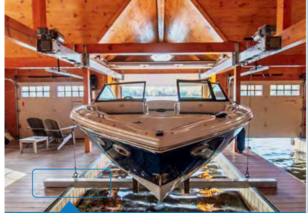
Bunk style cradle system with pull-out tubes in place for winter storage.
