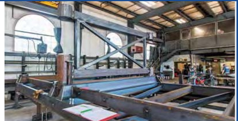
Underwater bracing during manufacturing.
