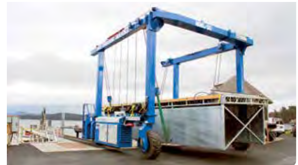
Above Left: Commercial marina system with wave attenuators incorporated into the dock system. Above Right Top: Wave attenuator section during final production in our shop. Above Right Bottom: wave attenuator section during initial installation.
