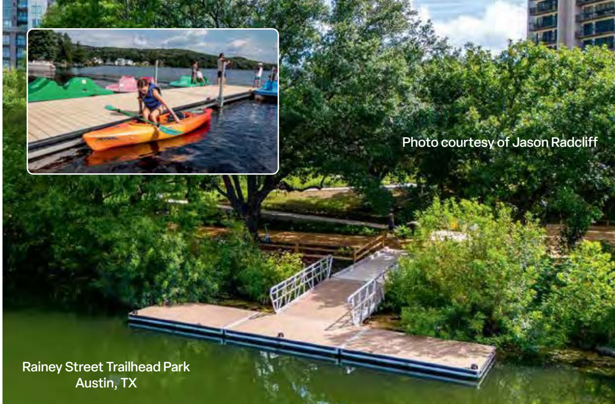
Aluminum floating "paddle" dock with low freeboard for easy entry for kayaks and other crafts.
