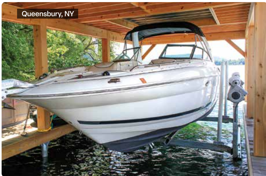
Above: 12,000 lb. capacity Ultimate Lift installed in a slip within a boathouse with standard vertical guides & upgraded oil bath drives.
