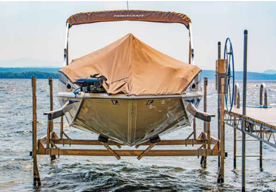
Above: 4,500 lb. boat lift manual handwheel.
