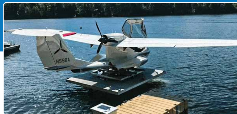
Seaplane lift utilizing a stock hydraulic lift with a custom turntable platform.
