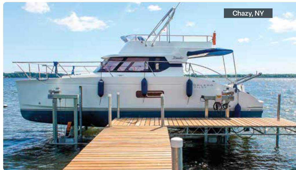
Above: 18,000 lb. capacity Ultimate Lift with custom bunks for catamaran hull.
