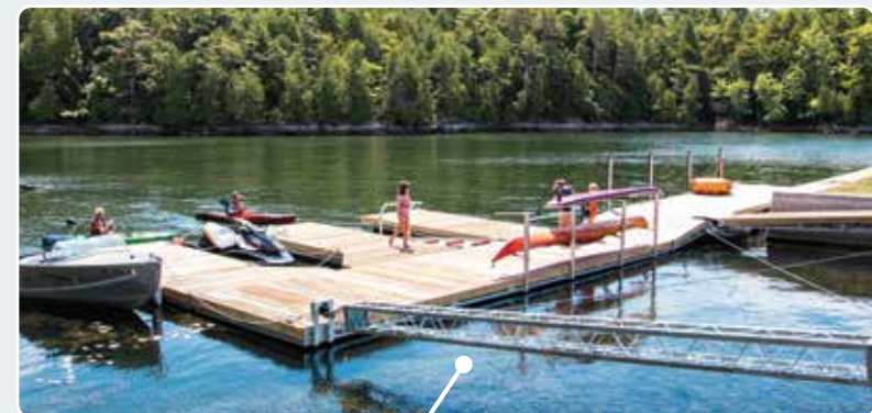
Stiff arm anchoring to eliminate any in-water anchoring.
