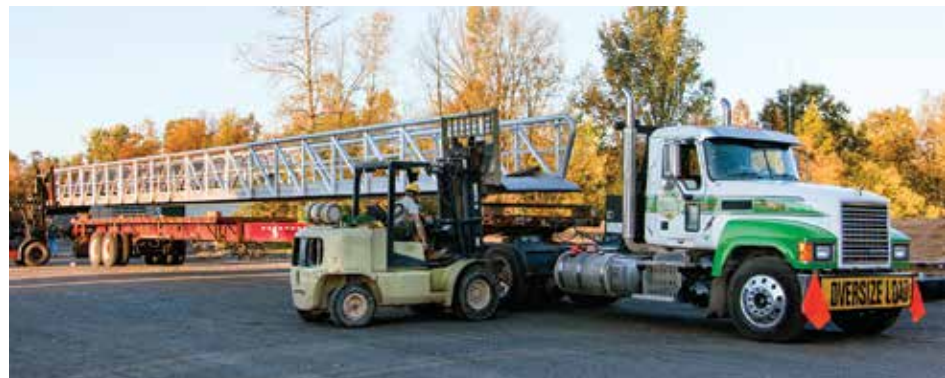
80' long gangway being loaded for delivery
