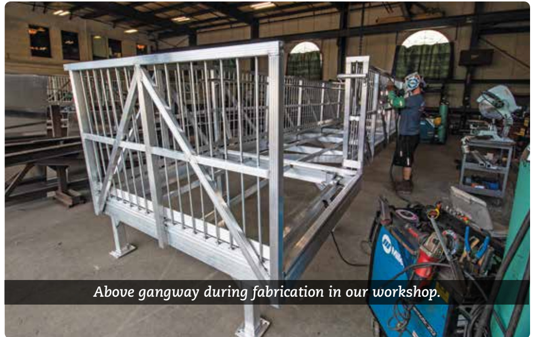
Above: Boarding gangway with spindle rail – gangway designed for ADA access to a high freeboard marine research vessel.
