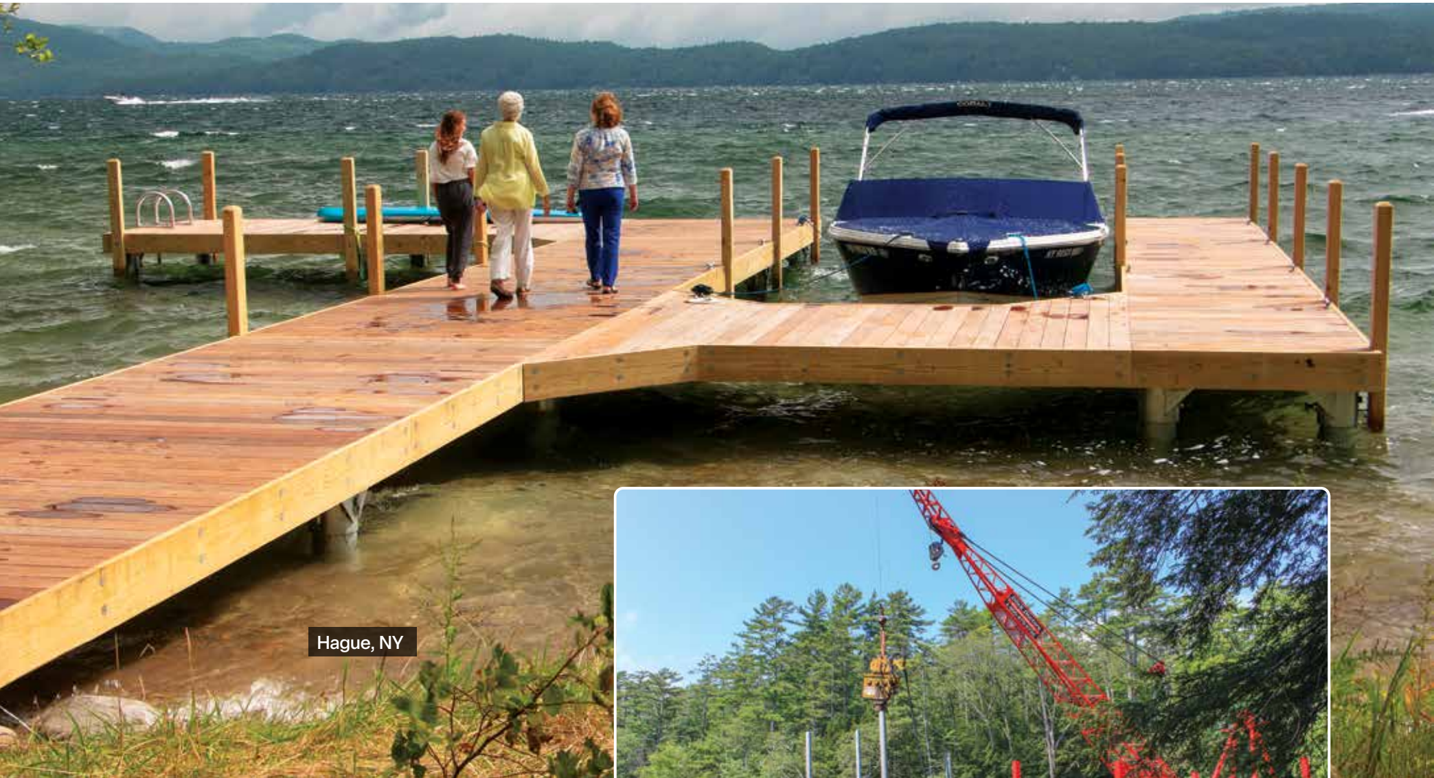
Above: U-shaped pile dock with Ipe hardwood decking.
