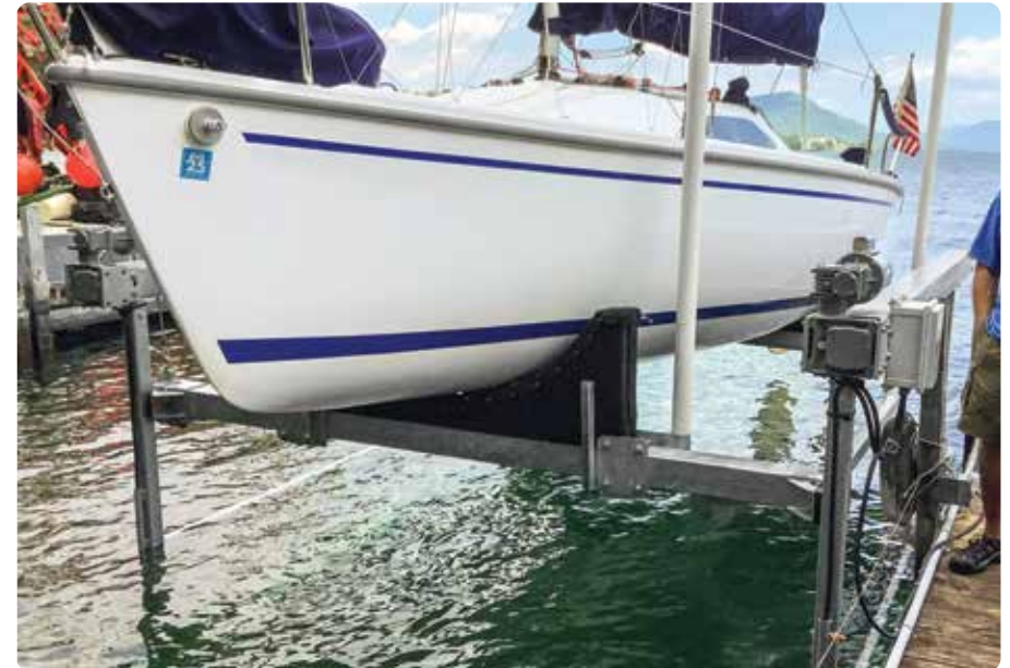
Ultimate 6,000 lb. boat lift with custom laminated timber/carpeted bunk upgrade to accommodate a shallow draft fixed keel sailboat.
