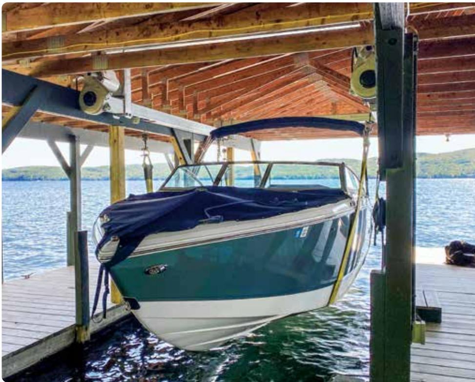
Above: Sling style system for shallow water applications.
