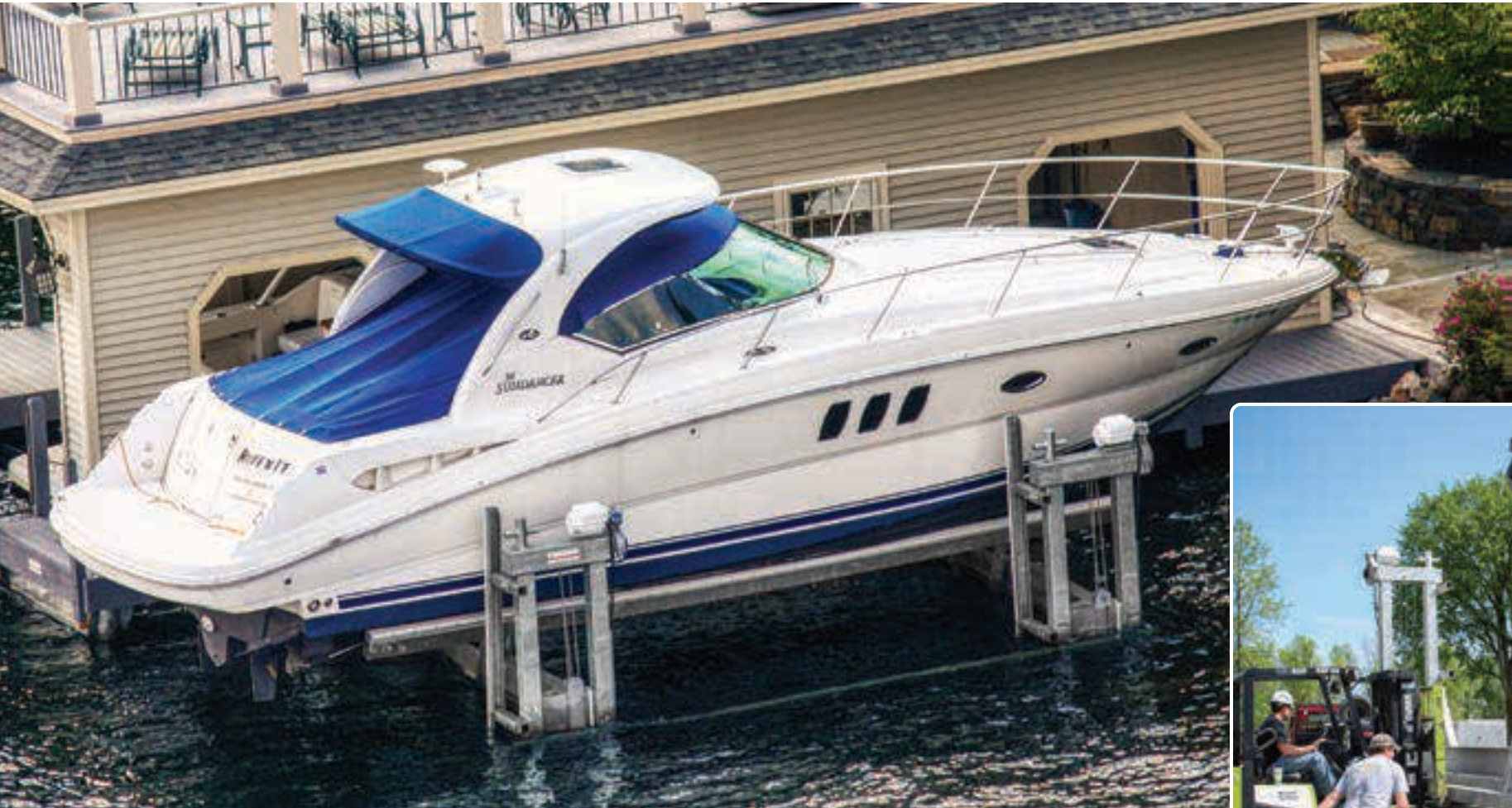
Above: 32,000 lb. capacity Ultimate Lift.
