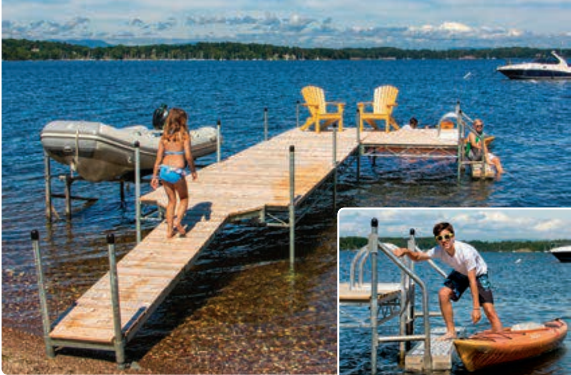
Above: 2' x 10' catwalk and 6' x 10' leg docks with cedar decking and 1,200 lb. vertical boat lift. Right: Lower access platform (see p. 14).
