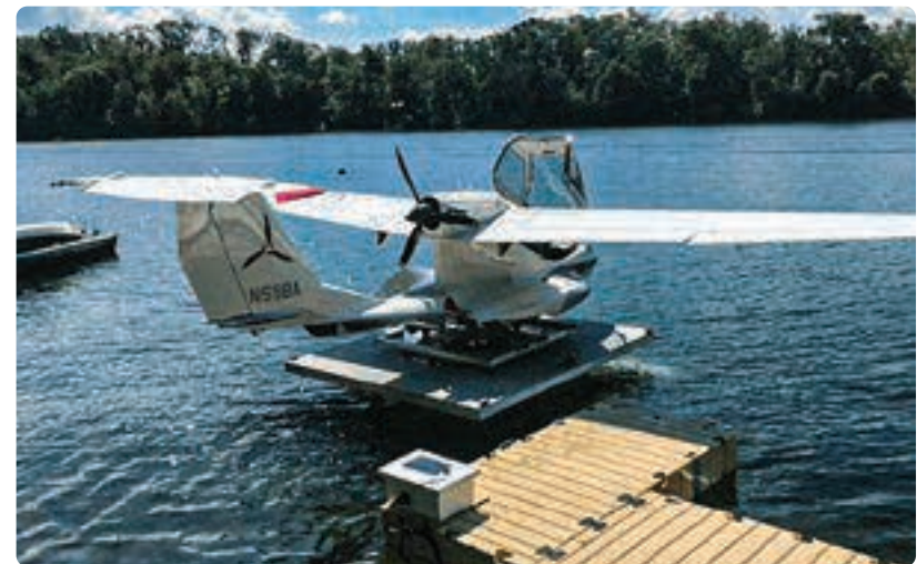
Seaplane lift utilizing a stock hydraulic lift with a custom turntable platform.
