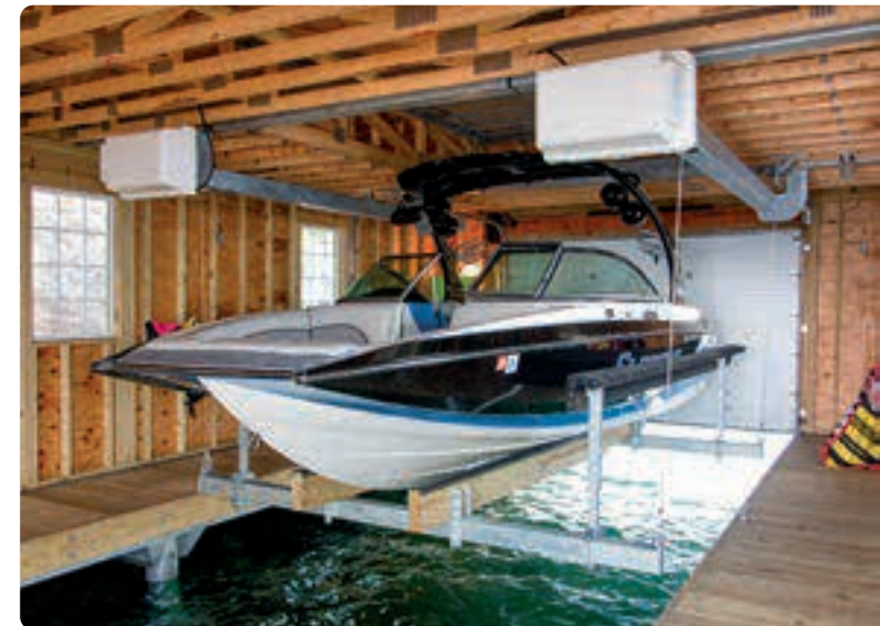
Boat lifted during the summer season with pull-out tubes retracted.
