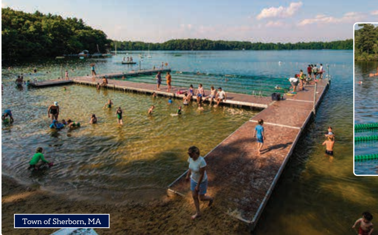
Left and Above: Heavy duty aluminum floating docks with composite decking and custom swim turn boards.
