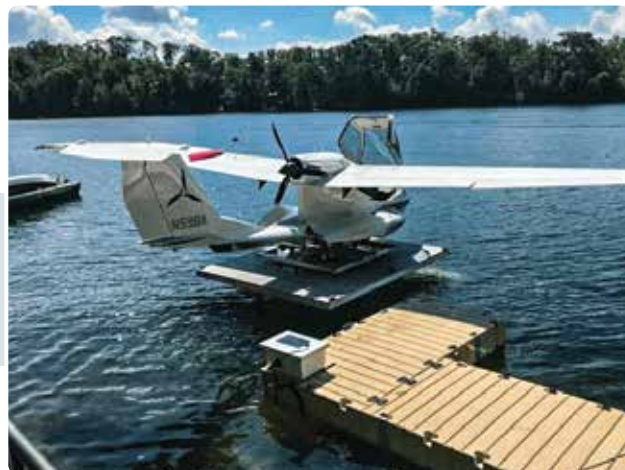
Seaplane lift utilizing a stock hydraulic lift with a custom turntable platform.
