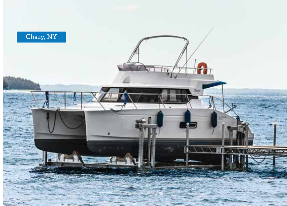
Above: 18,000 lb. capacity Ultimate Lift with custom bunks for catamaran hull.
