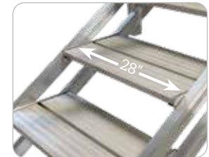
non-skid, 28" wide aluminum stair treads
