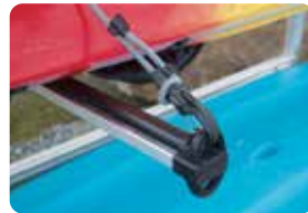
end caps with built-in tie-down openings
