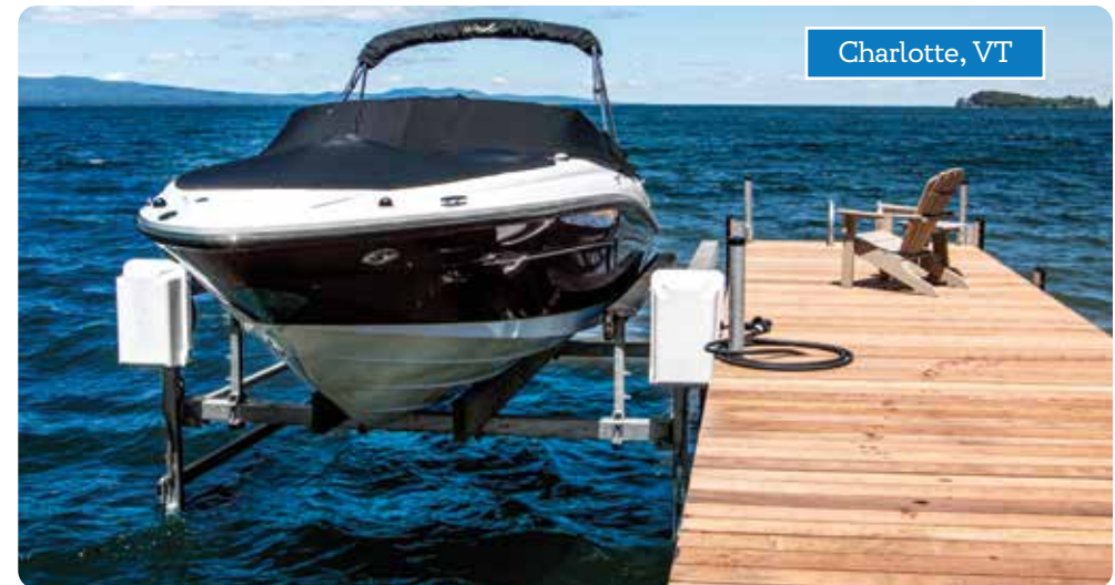
9,000 lb. capacity Ultimate Lift with standard flat plate AC drives.
