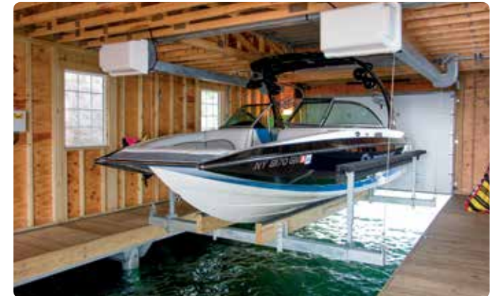
Above: Bunk-style cradle system with pull-out tubes in place for winter storage. Inset: Boat lifted during the summer season with pull-out tubes retracted.
