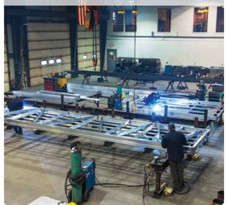
Aluminum docks being manufactured.
