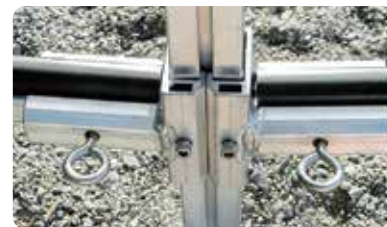
Support arms easily adjust along the main frame. Stainless eye-bolts for securing tie-downs on inside of craft.
