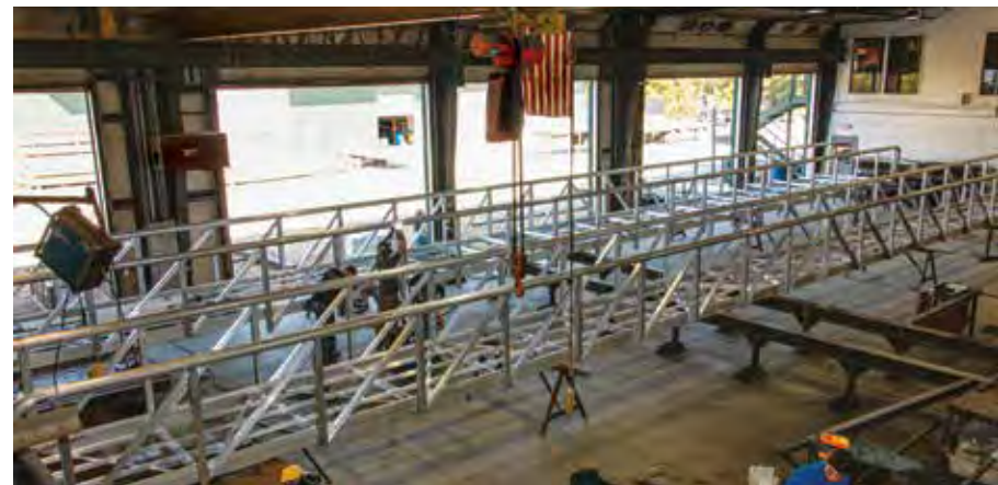
80' commercial aluminum gangway during production, then being loaded for delivery.
