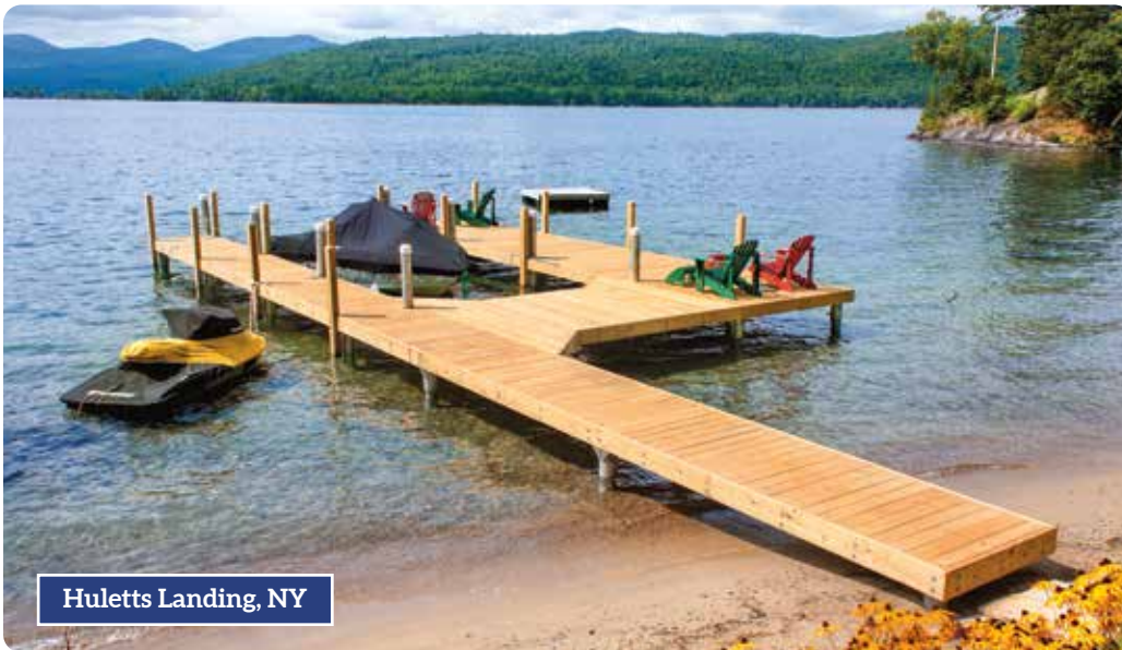
Above: Pile dock with piles extended above the decking.
