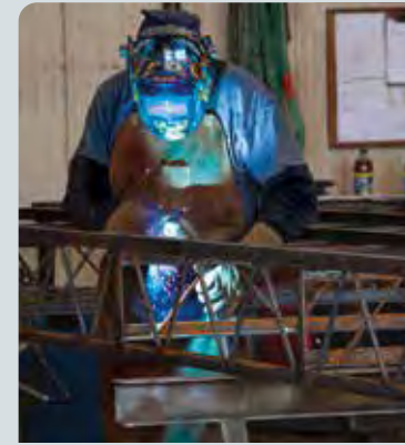
Above Left: Manufacturing of the dock frame. Above Right: Decking being applied in our workshop.
