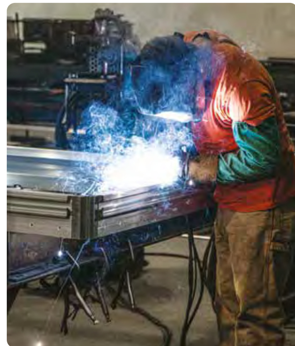
Aluminum docks being welded in our Ferrisburgh, VT manufacturing facility.
