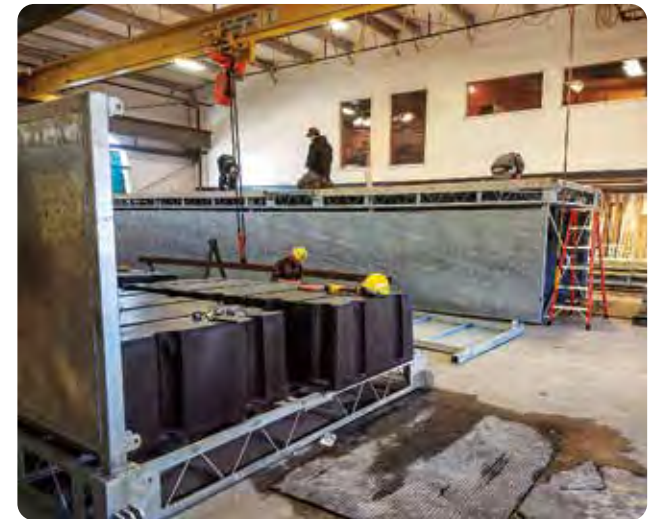
Above: Wave attenuators during production in our manufacturing facility.
