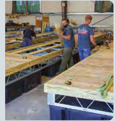
Above Left: Manufacturing of the dock frame. Above Right: Decking being applied in our workshop.
