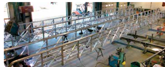
(2) 80' gangways during manufacturing.
