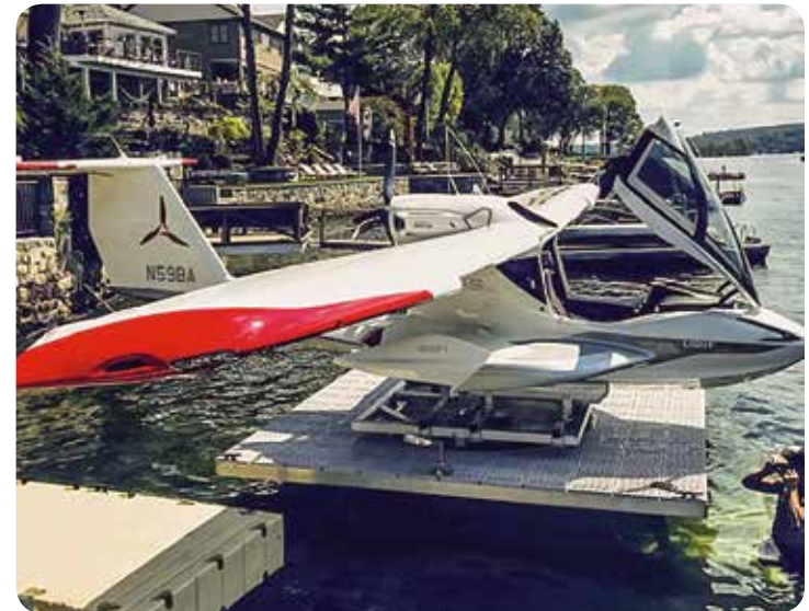
Hydraulic lift with custom platform & revolving bunk system to accommodate sea plane.
