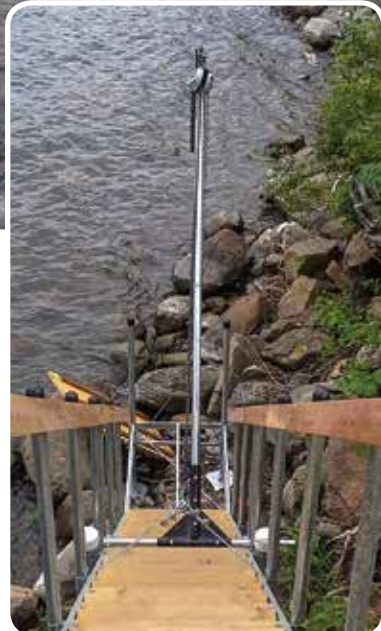
T-pole lift system in place ready to raise lower stair section for winter storage.
