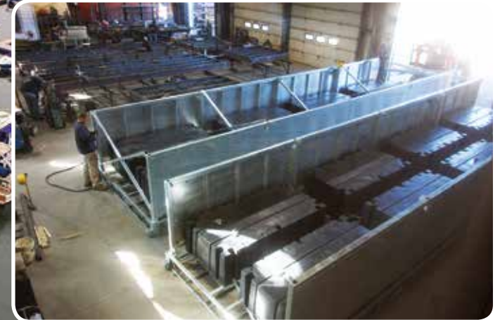
Wave attenuator in production facility having the flotation installed.
