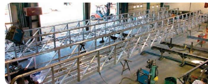
(2) 80' gangways during manufacturing.
