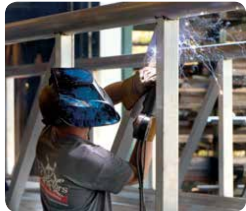
Manufacturing of an 80' gangway.
