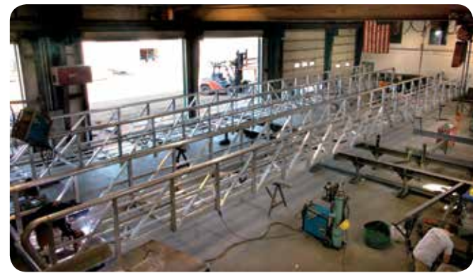
80' aluminum gangways during manufacturing.
