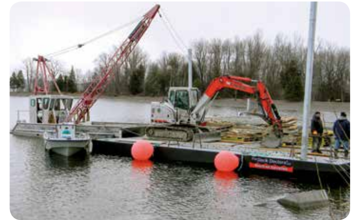
Portable Barge with Crane (above) or Excavator (below)
