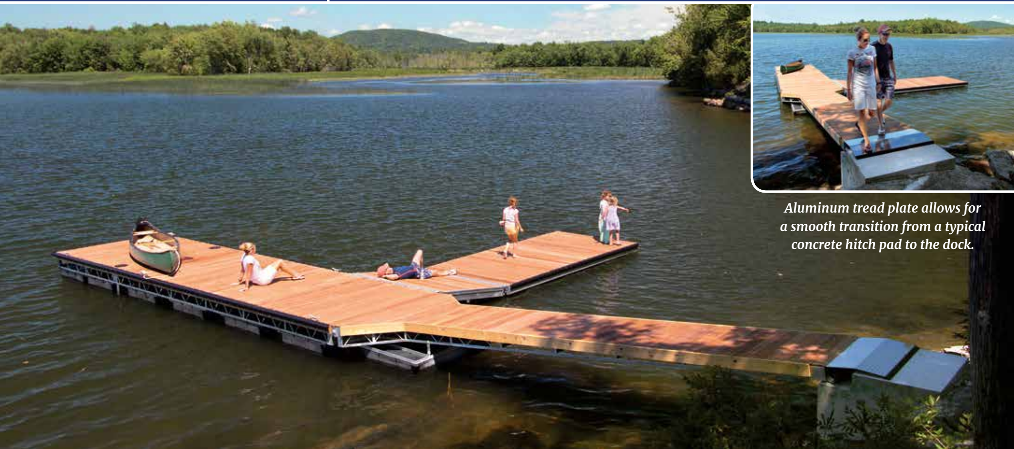
Steel truss floating dock with Ipe decking with lower freeboard heavy duty aluminum paddle dock extension.
