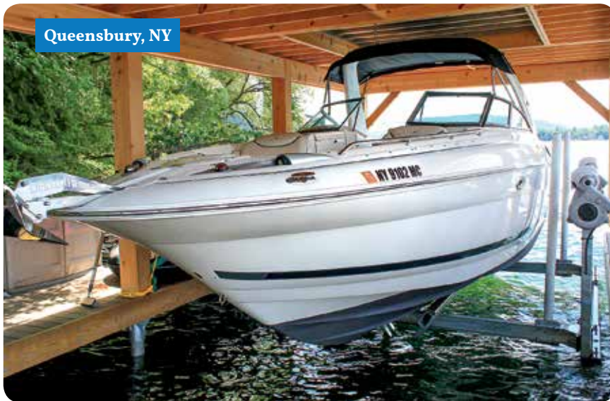
12,000 lb. capacity Ultimate Lift with oil bath drive upgrade.
