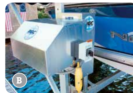
Direct A/C drive with manual switch
