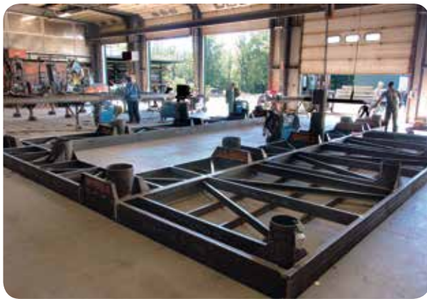
Pile dock being manufactured in our 25,000 square foot facility in Ferrisburgh, VT.
