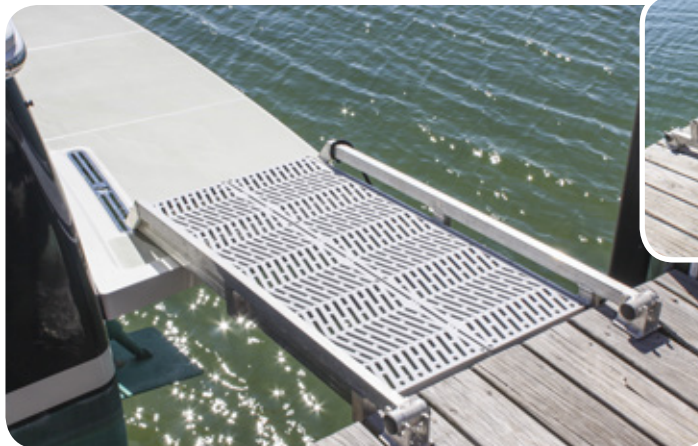
Left: Boarding ramp in boarding position.
