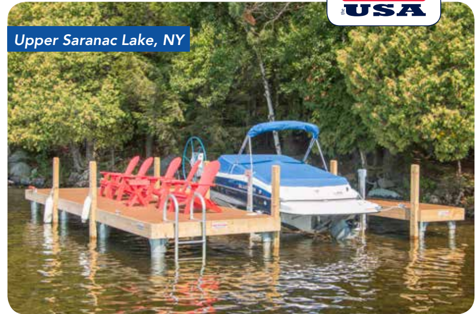
Pile dock with 8" diameter piles on outer supports for protection from ice on exposed side of dock.
