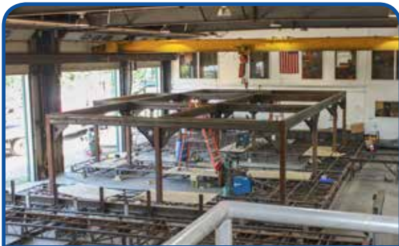
Above: Floating foundation and boathouse support structure during production in our shop.
