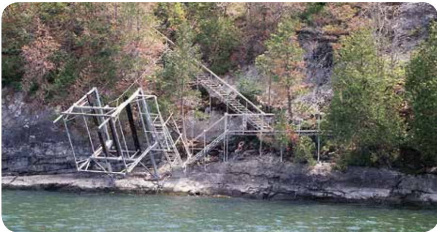
Above: The Dock Doctors Ultimate Lift (see pages 60-63) customized to attach to the shore with galvanized lift arms which allow it to be raised for winter storage.
