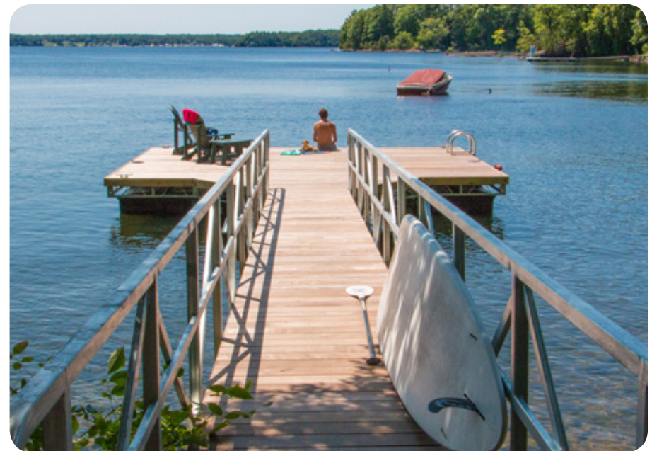
T-shaped floating dock with Ipe decking & truss skirt board.
