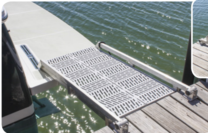
Left: Boarding ramp in boarding position.
