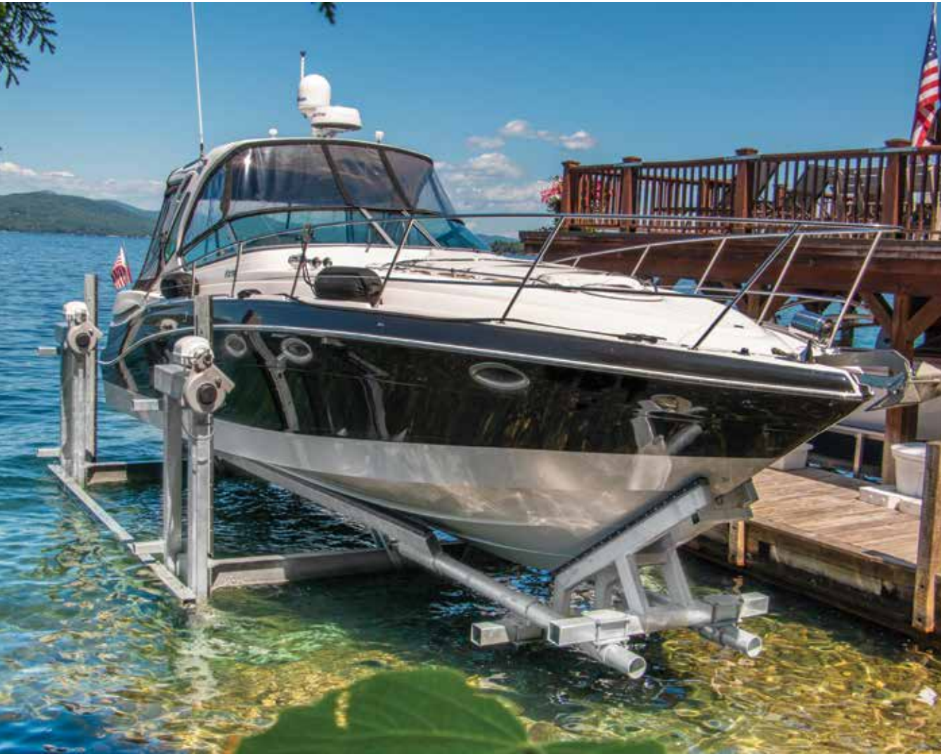
24,000 lb. capacity lift with front end bow stop, vertical guide-ons and optional oil bath drives.
