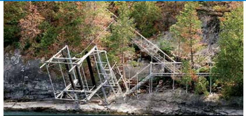
Our ultimate lift customized with galvanized lift arms allowing it to be raised for winter storage.
